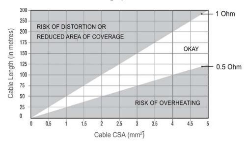
For example, to cover a room  $15m \times 10m (150m^2)$  the loop cable would need to be  $50m \log (2 \text{ sides } @ 15m \text{ and } 2 \text{ sides } @ 10m)$ . The recommended cable CSA for a loop this length is between  $1mm^2$  and  $2mm^2$ . Therefore, an amp which can cover areas of at least  $150m^2$  using  $1.5mm^2$  cable would be ideal.
